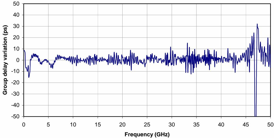
Aperture of group delay measurement: 81 MHz
