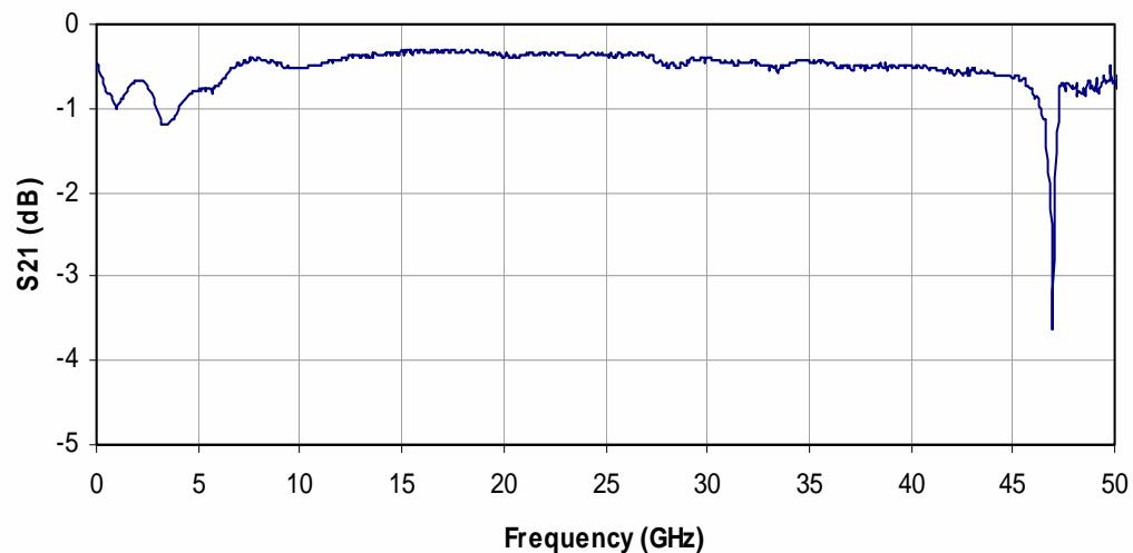
The spike at 47GHz is due to moding of the K connectors
