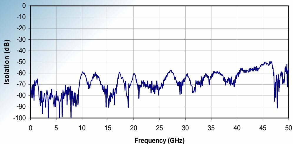
Measured between DC port and HF port.
